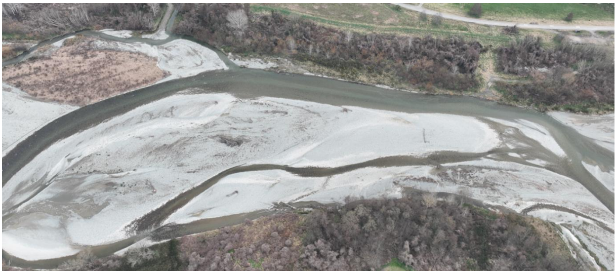
Figure C-2: River morphology during low flow. Note dynamic braiding pattern.
