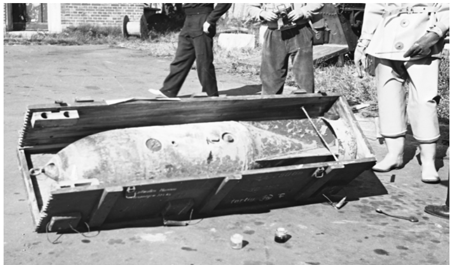
Figure 5: Washed/sailed ashore KC250 aerial mustard gas munitions shell in its original wood chest (Bornholm's Museum).
