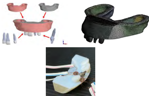
Figure 1. The left figure is the CAD models of maxillary bone (including cortical bone and cancellous bone), tooth and dental implant (including angled abutment
