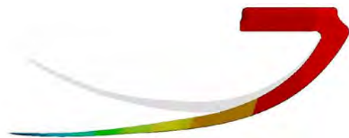
Figure 2: The mode shape of the first mode of vibration of an ESAR foot design.
