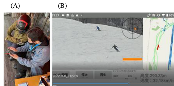
Figure 1 The mobile terminal used in this study feeds back a video with a sensor visualizer item to the subject (A : left figure). At this time, both smartphones are connected via Bluetooth and the sensor information is displayed in sync with the video. The right figure shows a part of the image displayed to the subject (B : right figure).
