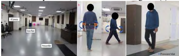
Figure 1 Data collection in (a) Gait & Motion Analysis Lab using (a)Wearable Sensor (b) Pressure Mat.
