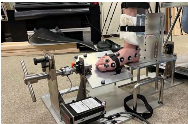
Figure 1 Measurement of midfoot passive resistance torque and three-dimensional foot kinematics.
