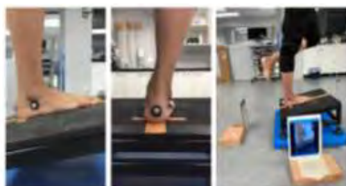
Figure 1 Marker placement below the lateral malleolus (left image) and on the heel (middle image). The back round sticker of 24 mm in diameter and retroreflective marker of 12.5 mm in diameter enabled tracking within the Calf Raise application and Qualisys SD motion capture system, respectively. The placement of two-iPad devices positioned 30 cm from the markers is also shown (right image).
