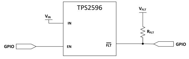
Figure 52. Single Device, Self-Controlled
