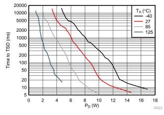
Figure 55. Thermal Shutdown Limit Plot
