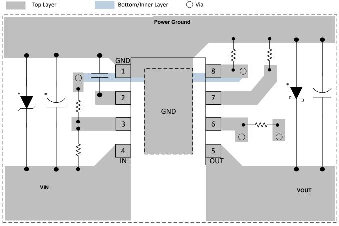
\* Optional: Needed only to suppress the transients caused by inductive load switching
