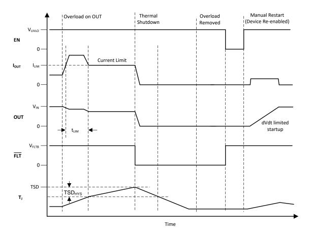
Figure 49. TPS2596x0 Overcurrent Response (Latch-off)
