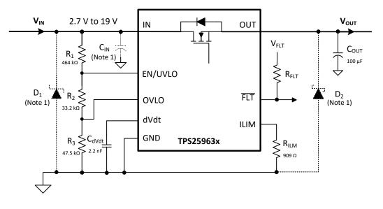
(1) C<sub>IN</sub> is optional and 0.1 μF is recommended to suppress transients due to the inductance of PCB routing or from input wiring. If system needs to pass IEC 61000-4-4 EFT test, minimum C<sub>IN</sub> of 1 μF should be used to prevent eFuse from turning off during EFT bursts.
