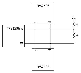
Figure 53. Multiple Devices, Self-Controlled
