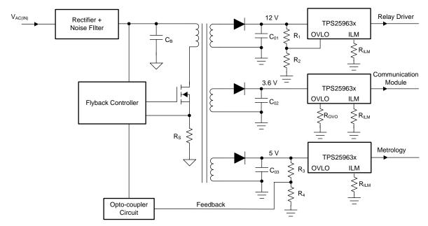
Figure 60. Energy Meter Power Rail Protection Example
