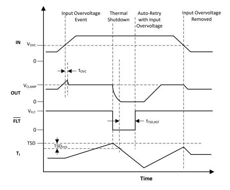
Figure 47. TPS25962x Overvoltage Clamp Response
